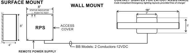
Typical Wiring Specification: UL AWM Style: Control Cable #20 AWG 300V
