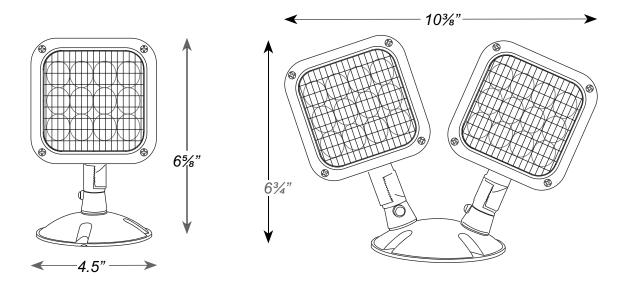
Heads can be rotated sideways (FIG. 6 & 7) by loosening the horizontal adjustment screw (FIG. 8) or tilted up/down by loosening the vertical adjustment screw (FIG. 9).
