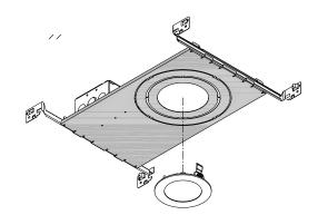
Pull the spring clip on the fixture up and through the ceiling hole.
