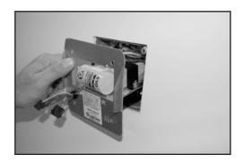
**3.** Connect polarized battery plug and install Base Plate Assembly into J-Box. Route AC wiring and wire nuts into space above battery.
