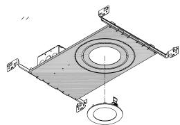
Pull the spring clip on the fixture up and through the ceiling hole.
