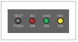
All MPS systems provide a monitoring panel on the front of the unit to show operating status. This panel provides a test switch for user initiated system tests, and a three-LED array that provides an intuitive visual indication of unit readiness.
